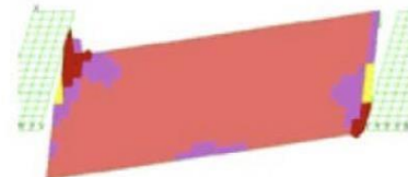
Figure 16-9: Limit equilibrium analysis of typical failure modes by Mitchell (1991)
