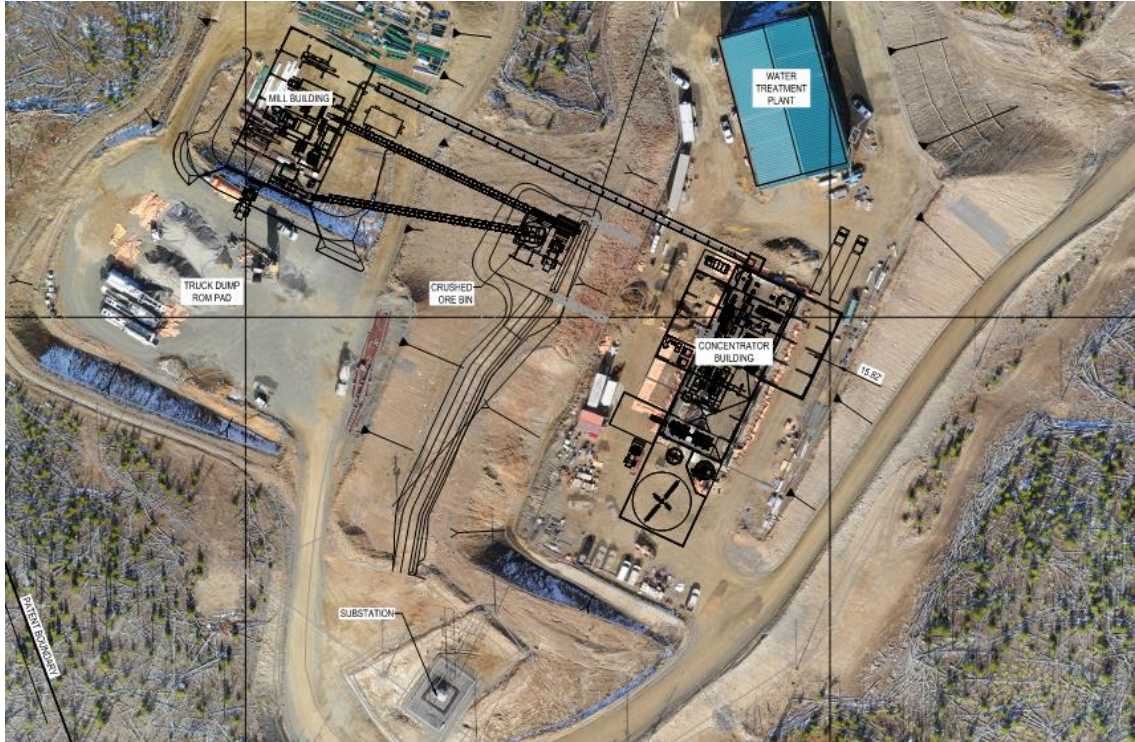
Figure 18-3: ICO Process Plant Layout
